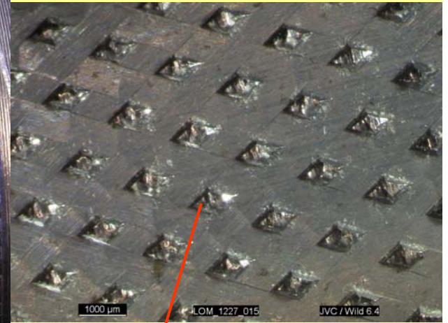
Cracked teeth; 1/3 of the top is missing: Contact to hard part.
