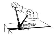
Bring the sealer handles completely together to assure a proper crimp.
