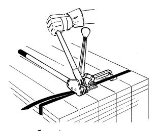
2. Bring sealer handles completely together to assure a proper notch.
